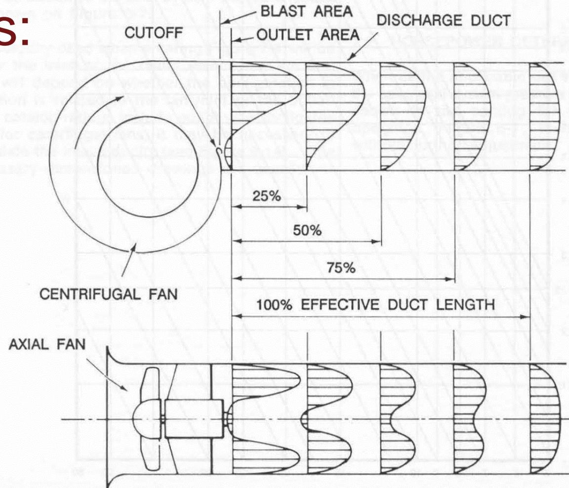
TO CALCULATE 100% EFFECTIVE DUCT LENGTH, ASSUME A MINIMUM OF 2-1/2 DUCT DIAMETERS FOR 2500 FPM OR LESS. ADD 1 DUCT DIAMETER FOR EACH ADDITIONAL 1000 FPM.
