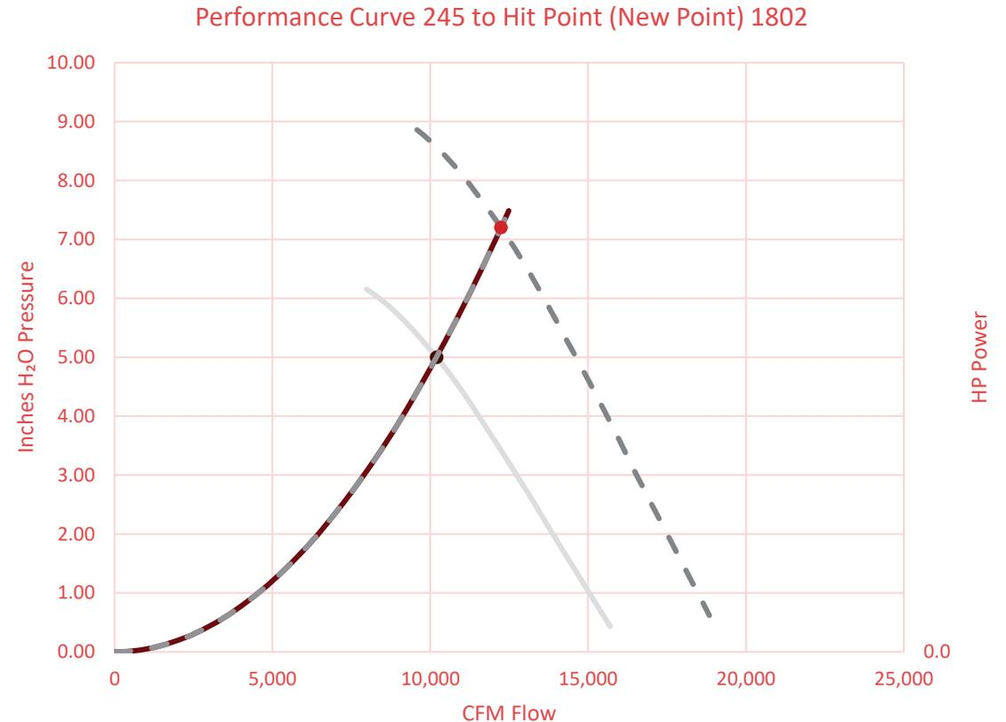
$$CFM_2 = CFM_1 * \left[ \frac{RPM_2}{RPM_1} \right] * \left[ \frac{K_1}{K_2} \right] \quad P_2 = P_1 * \left[ \frac{RPM_2}{RPM_1} \right]^2 * \left[ \frac{\rho_2}{\rho_1} \right] * \left[ \frac{K_1}{K_2} \right] \quad HP_2 = HP_1 * \left[ \frac{RPM_2}{RPM_1} \right]^3 * \left[ \frac{\rho_2}{\rho_1} \right] * \left[ \frac{K_1}{K_2} \right]$$
