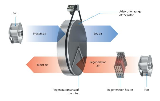
Desiccant drying - typical principle of operation
