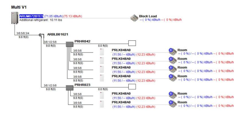
Here's an example of a Small AHU system in LATS-HVAC. The combination ratio should follow the rules in the combination ratio table (Table 6).
