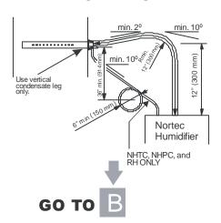
Figure 2: Distributor Above Humidifier
