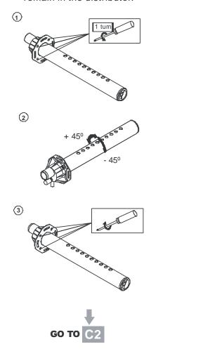
Figure 6: Vertical Airflow
