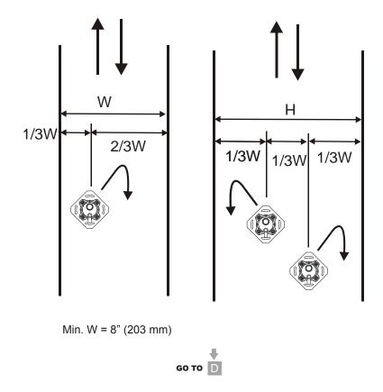
Figure 8: Vertical Airflow
