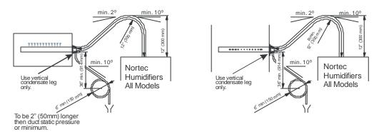
Figure 3: Distributor Below Humidifier
