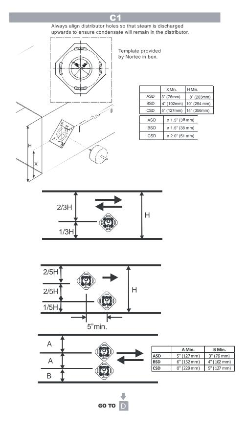
Figure 7: Horizontal Airflow
