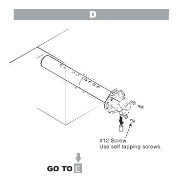
Figure 9: Distributor Mounting - Horizontal & Vertical Flow
